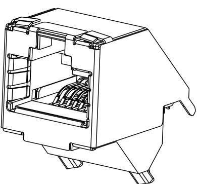
MATERIAL: HOUSING - HIG IR REFLOW SOLDERING PROC TERMINALS - 0.18MM THICK 3.81µm MINIMUM THICK MAT 0.76µm MINIMUM GOLD IN L ENTIRE TERMINAL PLATED W SHIELD - 0.25MM MIN THIC 1.27µm THICK NICKEL AND COMPENSATION PCB - FR-4. JACK CAVITY CONFORMS TO SUBPART F.
